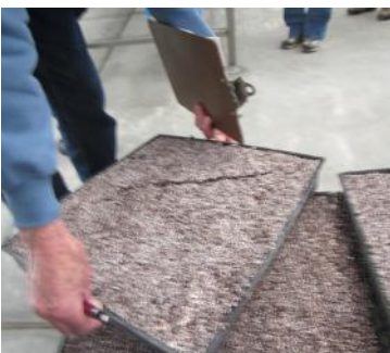
NOT like this! See the cracks opening?
